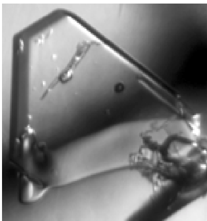
Figure 10b: Photograph of a 0.5mm near-surface faceted crystal harvested from the north-facing site on January 13 th .
