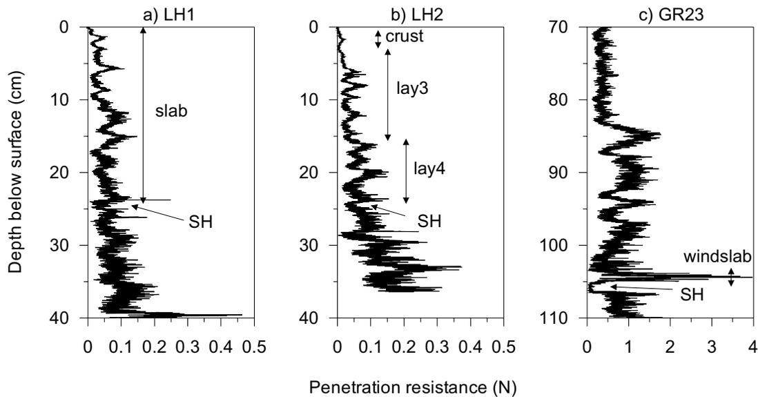
Figure 2: A “representative” SMP profile with the layers investigated for this research for a) LH1, b) LH2 and c) GR23. Note the different scales for the three profiles.
