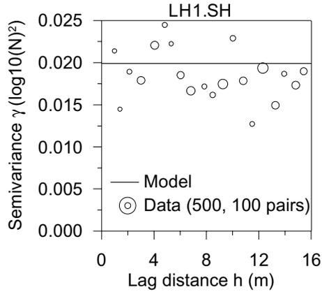
Figure 3: A pure nugget variogram model best fit the penetration resistance for the surface hoar layer at Lionhead 1 (LH1.SH).
