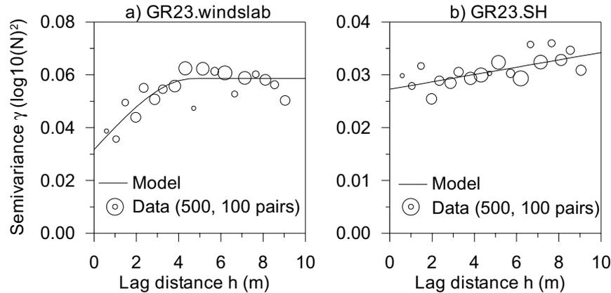
Figure 5: At the Swiss site a) a spherical model provided the best fit for the slab (GR.windslab), and b) the buried surface hoar layer (GR.SH) was best fitted with a linear model plus a nugget.
