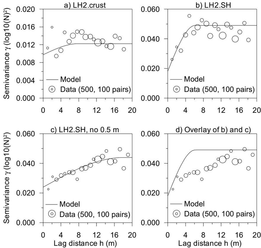
Figure 4: We fit a spherical model to the penetration resistance of the a) crust layer (LH2.crust) and the b) surface hoar layer (LH2.SH) at Lionhead 2. When the 0.5 m grid is removed from the Lionhead 2 data, the semivariogram changes significantly (c). d) shows the modeled semivariogram for all the Lionhead 2 data, with the data points for the data with the 0.5 m grid removed to emphasize the difference when the fine grid is removed.
