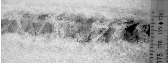
Fig. 6. A close-up photo of the double surface hoar layers at the Lionhead site, taken prior to the collapse. The ruler is marked in centimeters.
