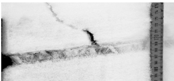
Fig. 7. Close-up photo of the tensile crack and collapsed surface hoar, taken shortly after the collapse. The ruler is marked in centimeters.
