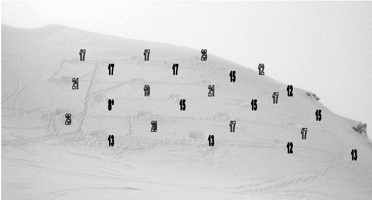
Figure 2: Photo from day two at Broken River, showing the day two CT results (in grey) and the remnants of the day one CT results (in black) in between and below the day two grid, illustrating the 10m spacing in the grid, and the 5m offset layout (up slope and to the left) for the second day. The * represents a CT result on a different layer. (Photo: Irene Henninger, Broken River / Yellowstone Club Patroller).
