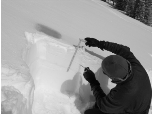
Figure 1: After applying dye, the author marks the slope parallel cuts that are conducted 10 minutes after dye application. Photo by Karl Birkeland.
