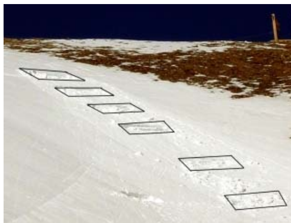
Figure 3: ECT300 results in the morning (with a frozen snow surface) show that all but three of our initial tests fully propagated across the 300 cm wide column (ECT300P). Interestingly, when we repeated those three tests in the afternoon (with a wet, melting snow surface), a fracture fully propagated across the entire 300cm column in all three tests. At this site we also conducted three standard sized ECTs in each of the six pits in the morning. All 18 of those ECT tests fully propagated across the column (ECTP).
