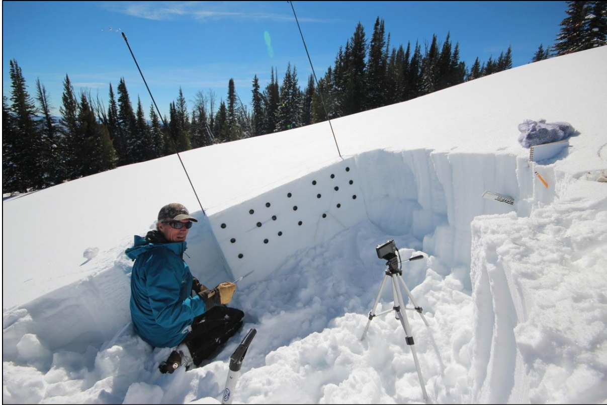
Figure 1: Our experimental setup involved taking high-speed video of our tests for particle tracking velocimetry. This picture also shows the relatively uniform, gently sloping meadow where we conducted our experiments.
