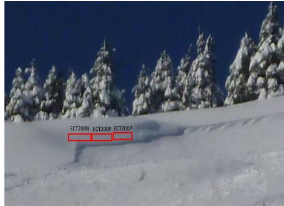
Figure 1: Test layout shows a series of ECT200 along an avalanche crown wall. We started from the center side of the avalanche and toward the flank until ECT200 result changed from ECT200P to ECT200N.
