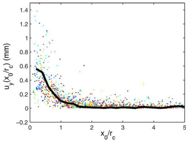
**Fig. 6.** Slope normal displacement  $u_y$  with normalized distance  $x_0/r_c$  for all 222 tests (each color represent one test) at the critical cut length  $r = r_c$ , i.e. the onset of crack propagation. The mean slope normal displacement of all experiments is depicted by the thick black curve.
