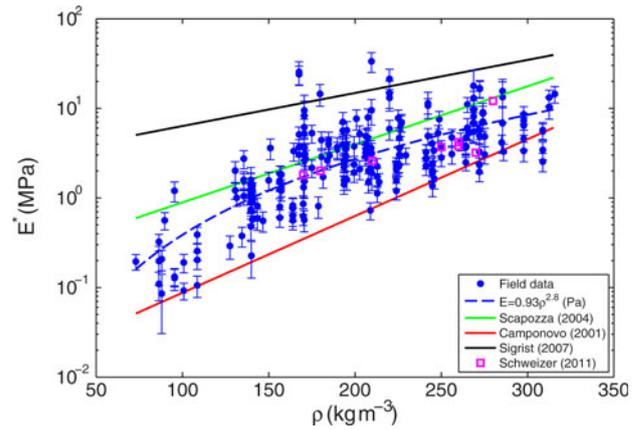
**Fig. 8.** Effective elastic modulus  $E^*$  with slab density. Field data (blue dots) and power law fit (blue dashed curve). Also shown are the parameterizations from laboratory studies presented in Scapozza (2004) (green line), Camponovo and Schweizer (2001) (red line) and Sigrist (2006) (black line) as well as estimates from SMP measurements (squares) from Schweizer and others (2011).
