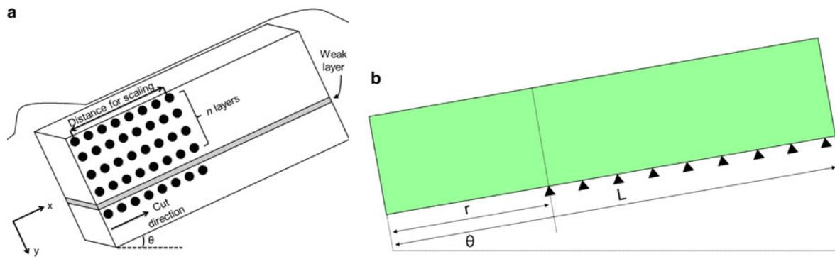
**Fig. 1.** (a) Schematic representation of the experimental setup and coordinate system used in the analysis with  $x$  the slope parallel direction,  $y$  the slope normal direction and  $\theta$  the slope angle. (b) FE model setup with a snow slab of total length  $L$  unsupported over the crack length  $r$  and rigidly supported at the base along the remaining length  $L-r$ . Triangles indicate fixed nodes.
