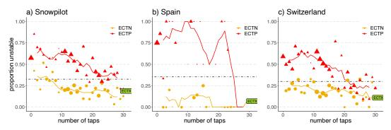
Figure 2: Proportion of unstable ECT locations for each combination of fracture propagation and number of taps until failure for the three data sets. The Snowpilot (a) and Swiss (c) results, which are based on a large number of ECT, look rather similar. In contrast, the ECT data from Spain discriminates better between ECT results indicating instability and stability, but also a much more random behavior due to the small number of ECTs.
