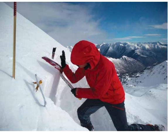
Jordi Gavaldà, avalanche forecaster at Val d'Aran avalanche center, performing an ECT at Montanyó d'Arreu in the Catalan Pyrenees (Spain). The ECT results were moderate to hard ECTNs. This agreed well with other observations made on this day, indicating a good bonding of the wind slab, which had formed during a storm several days earlier *Photo I. Moner.*
