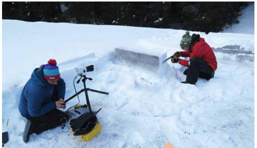
Figure 7: The third talk in the session investigated changes in PST critical crack lengths following loading. Karl Birkeland prepares to cut a PST while Basti Bergfeld films the test with a high-speed video camera at 3000 frames per second. Photo Alec van Herwijnen
