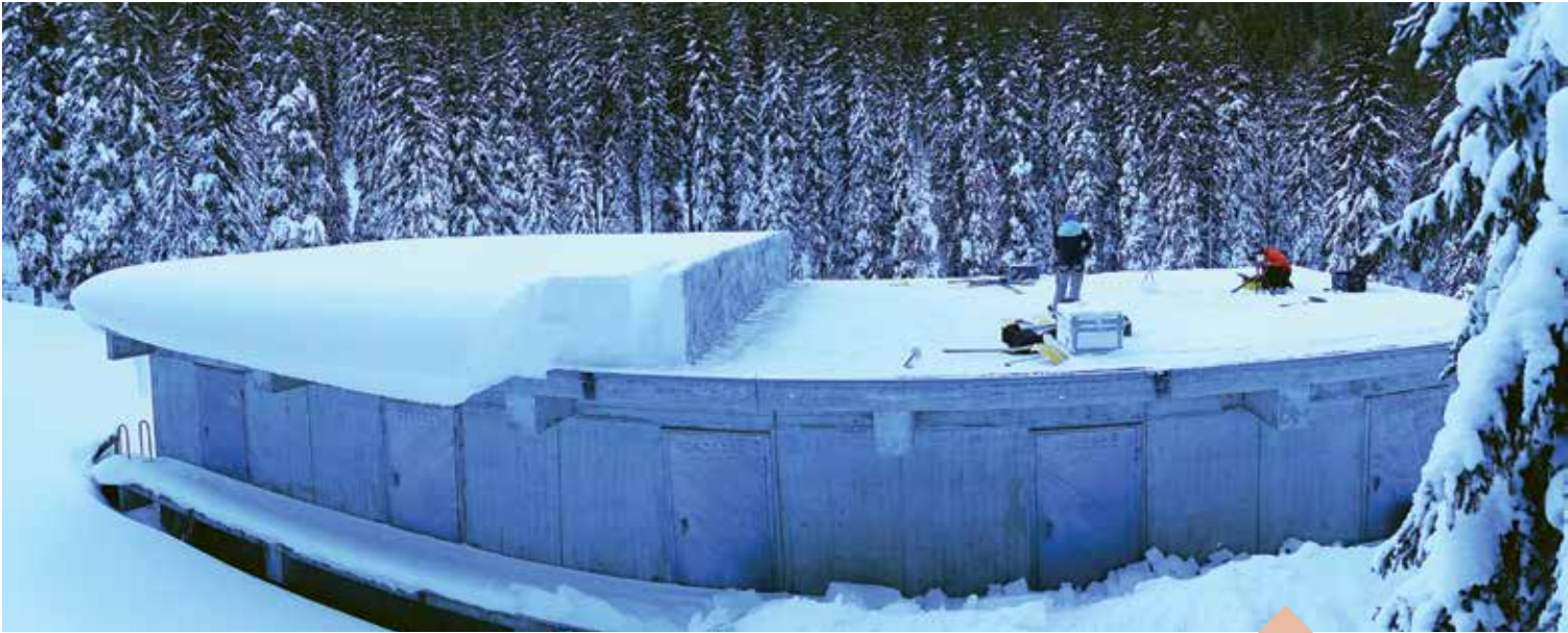
Figure 4: To better understand avalanche release, Basti Bergfeld and colleagues conducted extra-long Propagation Saw Tests (up to 10 m long) on top of a concrete bunker outside of Davos, Switzerland. Photo Alec van Herwijnen
